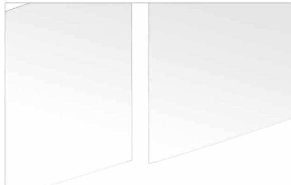
Lay absorbers with a gap of up to 20 mm
