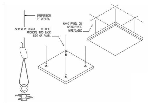
Utilising Rotofast Anchors simply hang your cloud or cube with 1.5mm stainless steel rope & a ziplock adjustor to achieve the correct height.
